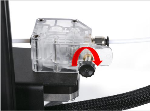
If the melted filament is not smooth, please increase the extrusion force by rotating clockwise.
