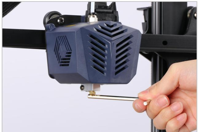
3. When the calibration succeeds, the machine will home and preheat the print head and heated bed (If you manually heat them up to the target temperature before leveling, the preheating will be skipped automatically). When the machine reaches the target temperature, it will probe 16 spots on the platform automatically.
